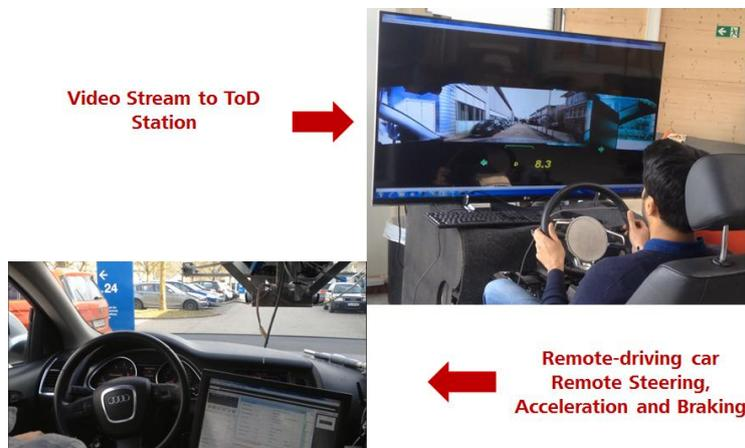
**Figure 6-8. Tele-Operated Driving Research Platform**
